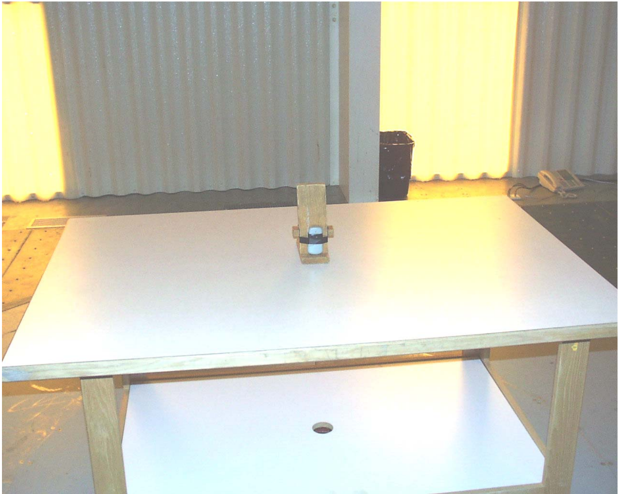
Photograph 1 - View of the Radiated Emission Test Setup (Vertical Alignment)
