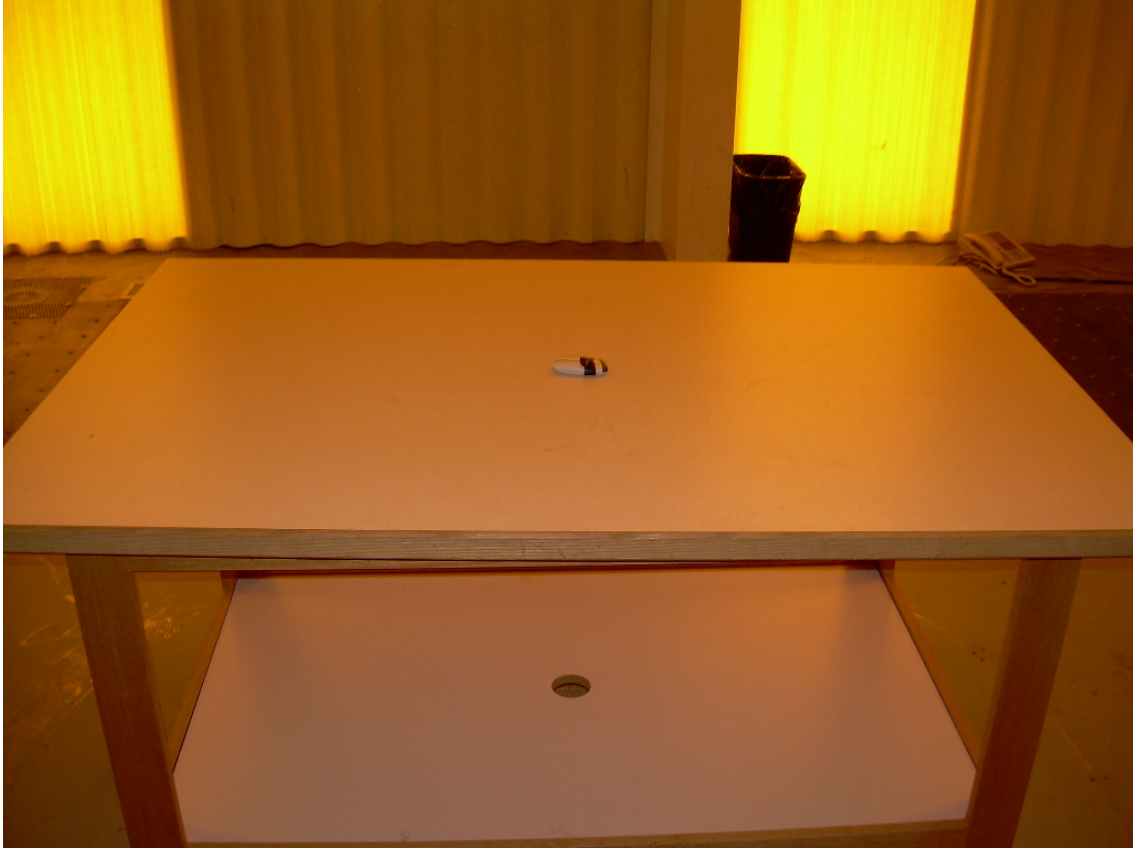
View of the Radiated Emission Test Setup (Horizontal Flat Alignment)
