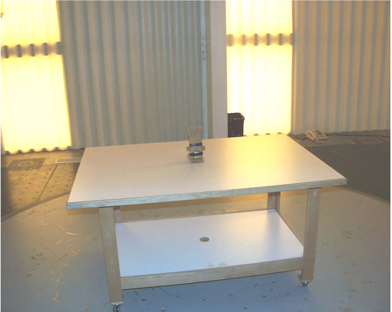
View of the Radiated Emission Test Setup (Vertical Alignment)
