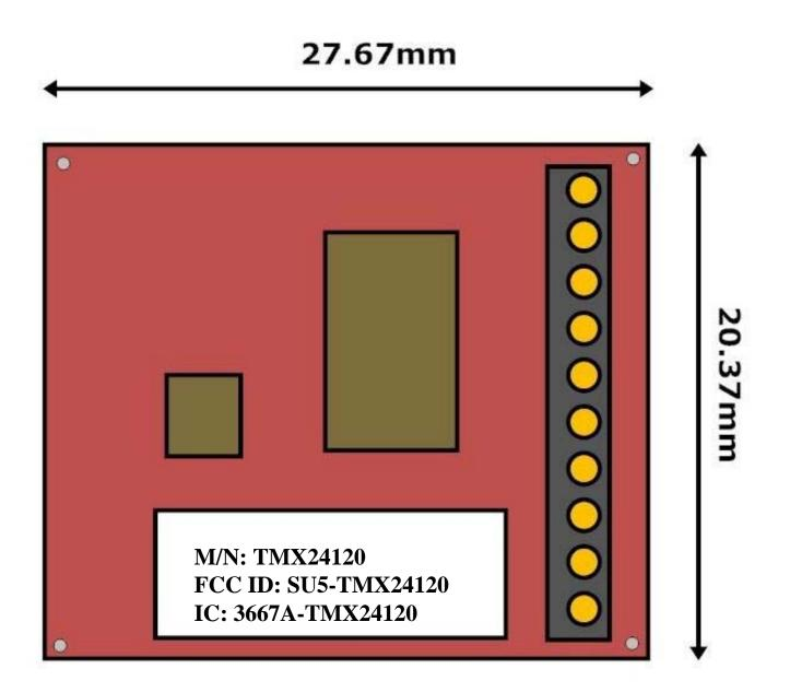
FCC & IC Label for Exterior Placement
