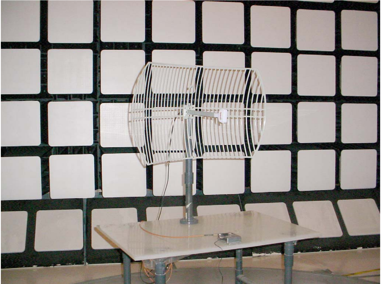
Radiated Emissions at 3 m EUT with 24 dBi Parabolic Antenna
