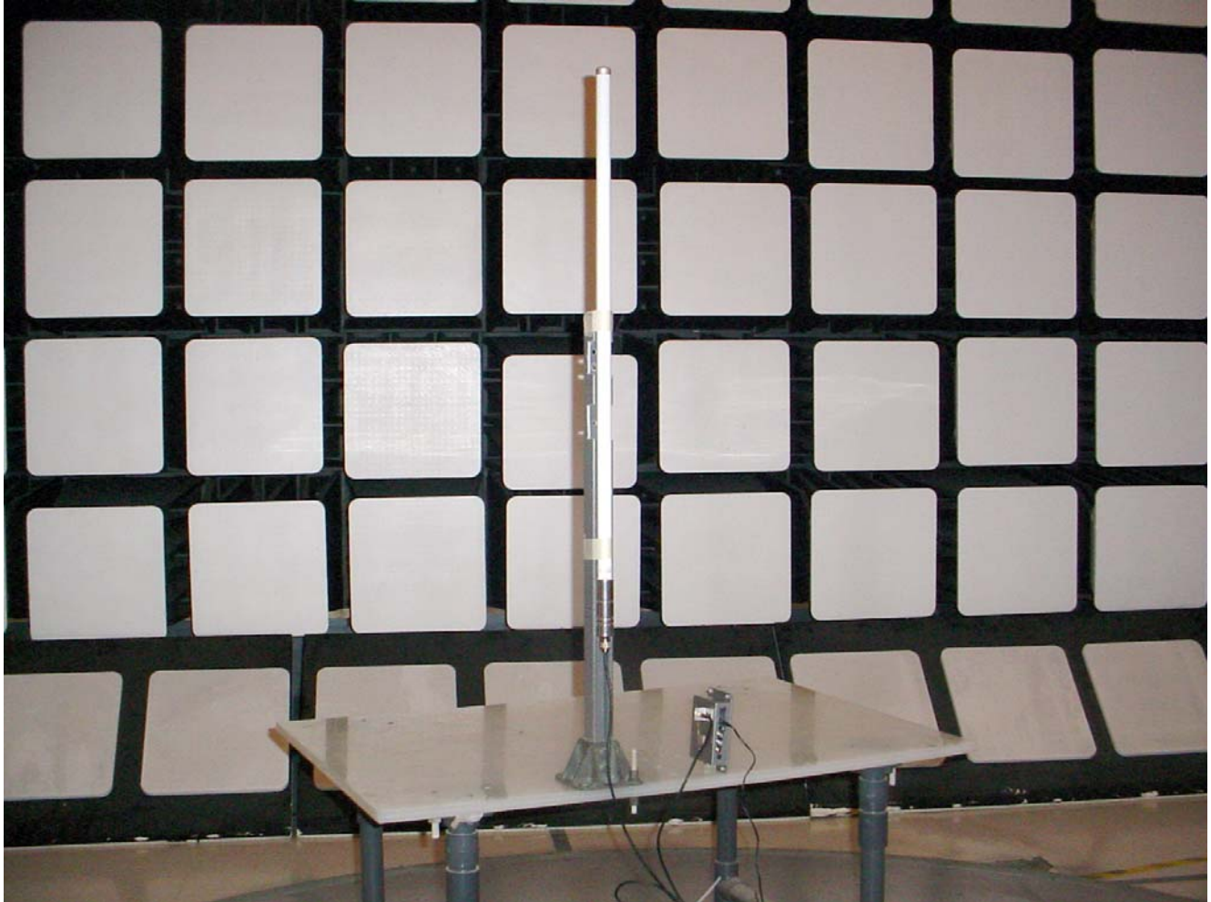
Radiated Emissions at 3 m EUT with 12 dBi Omni-directional Antenna (Orthogonal Position 2)
