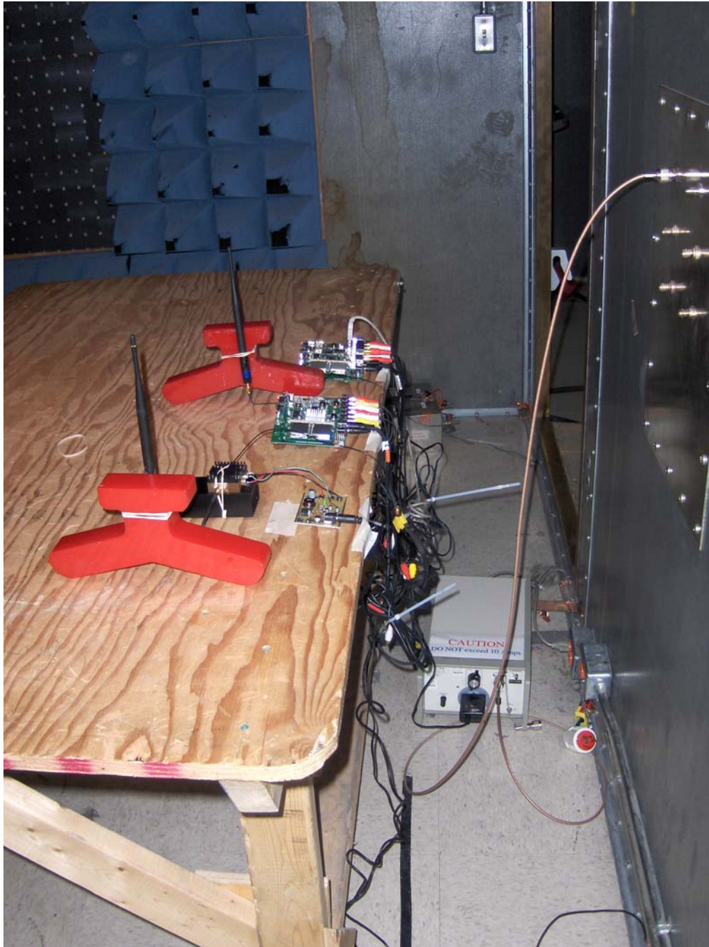
Power Line Conducted Emissions Test Configuration 2: EUT on Server (Master) and as Client (Slave) with Amplifier (Test Conducted on Power Source of the Test Jig Boards and Amplifier)
