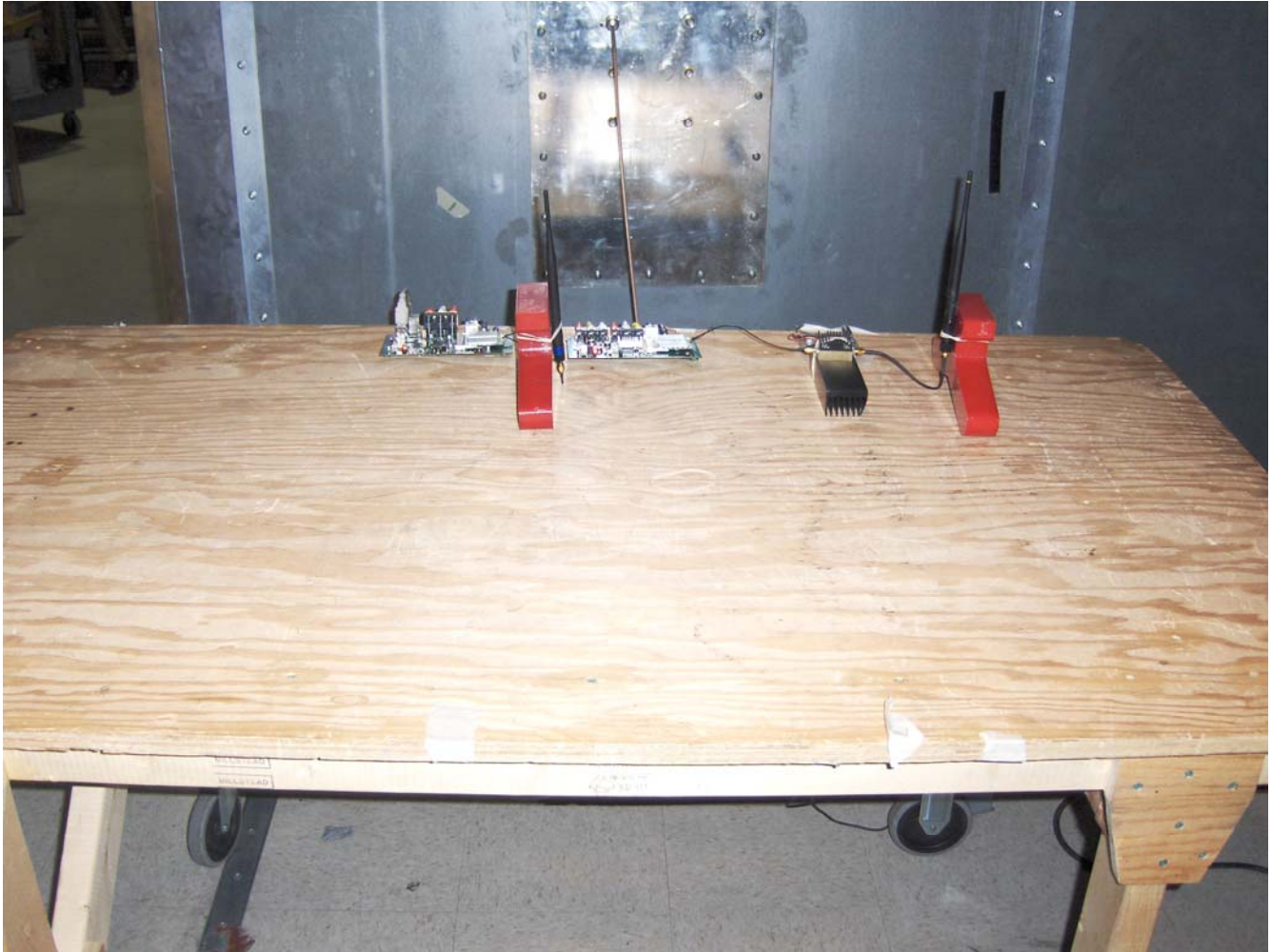
Power Line Conducted Emissions Test Configuration 2: EUT on Server (Master) and as Client (Slave) with Amplifier (Test Conducted on Power Source of the Test Jig Boards and Amplifier)
