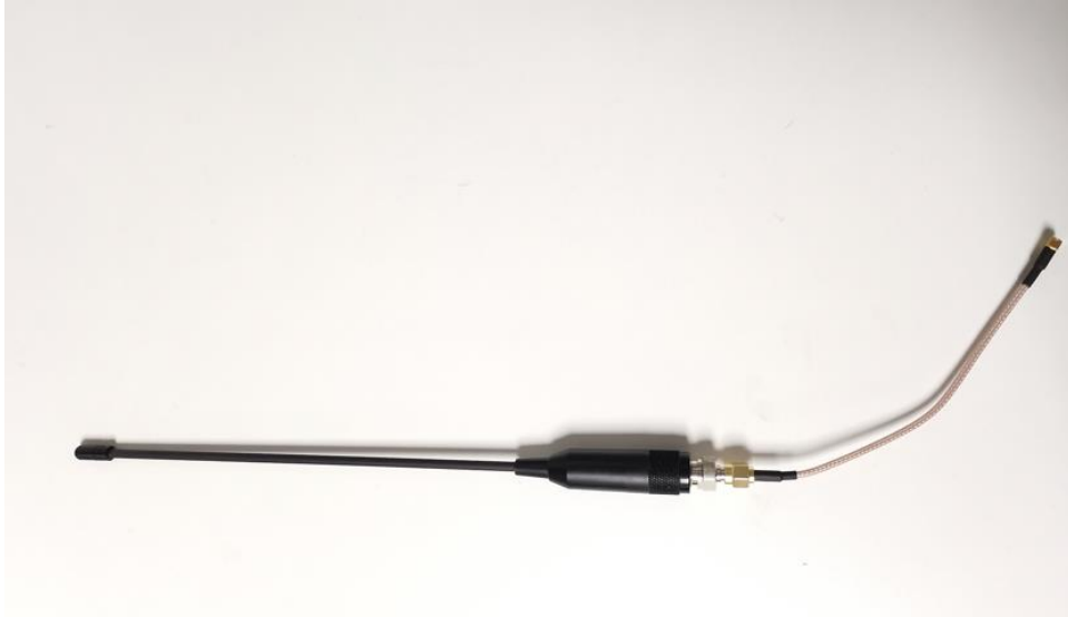
Antenna 4: dipole antenna, RP-N connector, 3dBi
