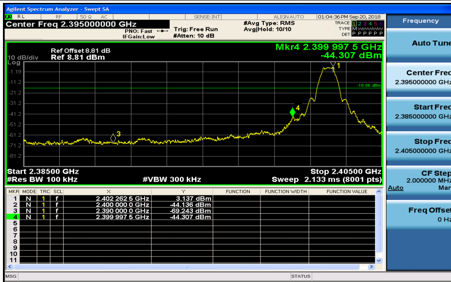
Band-edge for RF Conducted Emissions_BLE_2480_Hopping Off
