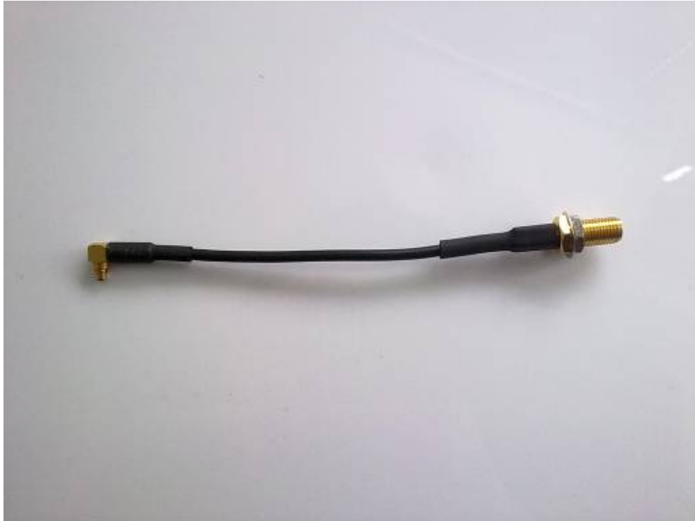
RF cable between EUT and Omnidirectional Antenna
