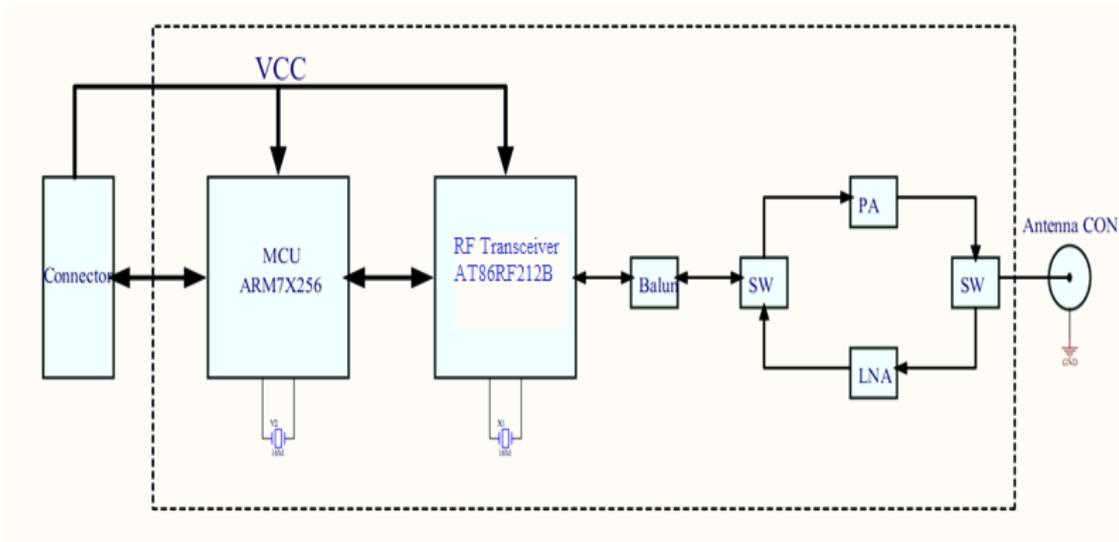
The module contains Atmel's AT91SAM7X256 Microcontroller, AT86RF212B RF transceiver, balun, two RF switches, power amplifier and low noise amplifier.
