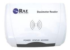
pass-by and short range data exchanges in a wireless manner, forconfiguring, activating, and diagnosing the dosimeters via the PC-installedsoftware, ProRAE Dosimeter V2.00 or higher versions. The PRR-1 has three visual indicators for showing its operation statuses and a USB port for enabling data exchanges with PC via a USB cable. In addition, it also has bolt-head receiving and slip-resistant features for being mounted on wall or reducing slippery when placed on a desk surface.
