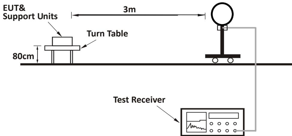
For Radiated emission 30MHz to 1GHz:
