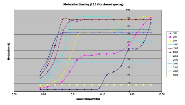
(d) A curve or equivalent data that shows that the equipment will meet the modulation requirements of the rules under which the equipment is to be licensed.
