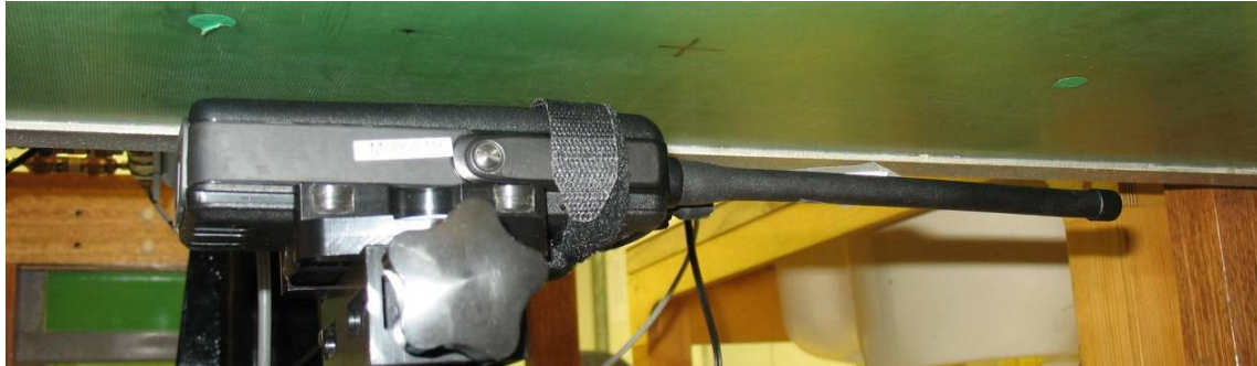
Face Frontal Position with 182mm Antenna
