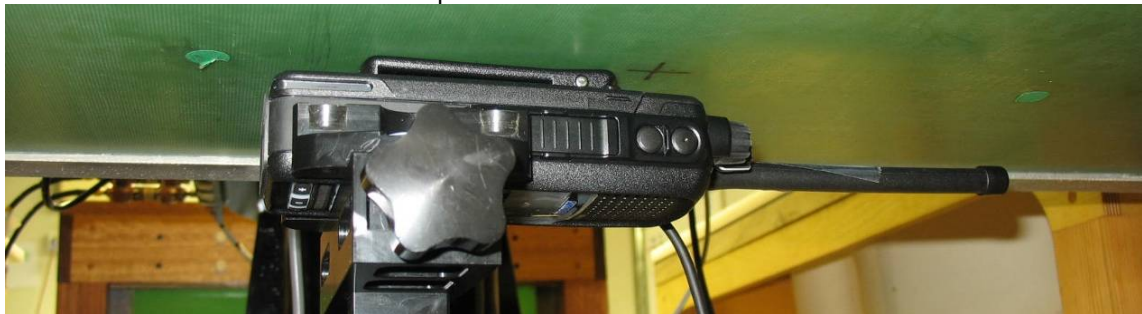
Belt Clip Position with 140mm Antenna
