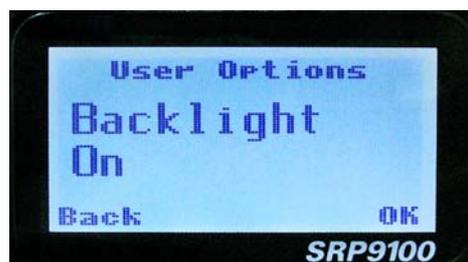
When the Function is selected, the function can be toggled ON or OFF with the “OK” key.
