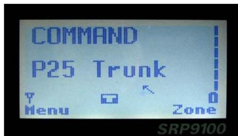
Trunked mode is indicated by the
