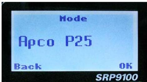
From the “**Mode**” menu, use the ▼ and ▲ keys to select the required operating mode, such as APCO P25, PMR or MPT Trunking. While the required mode is displayed, press OK to select that operating mode. The radio will then display the default screen for that mode.
