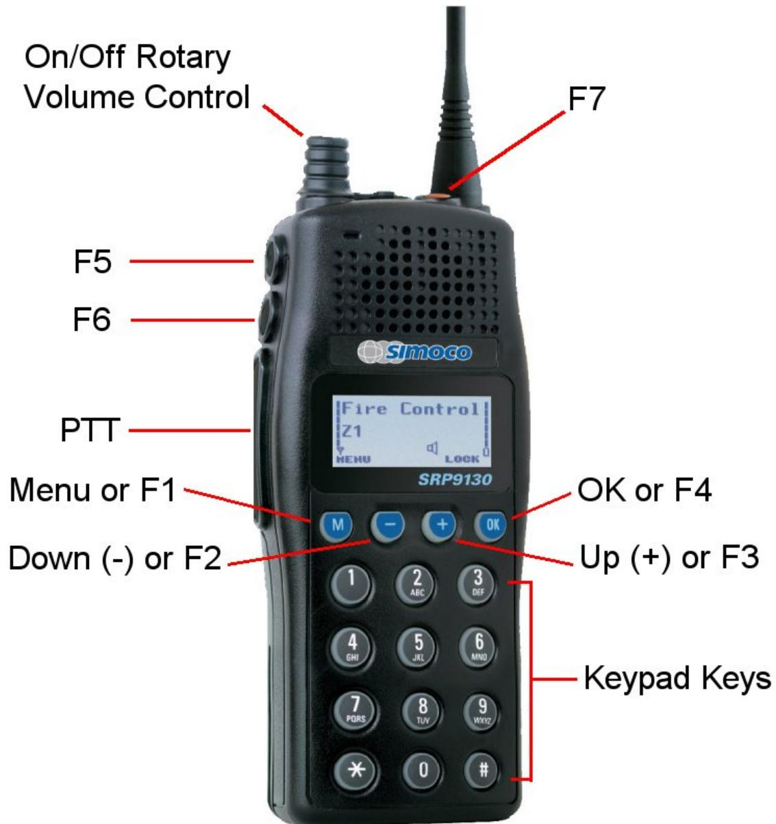
Figure 1 – SRP9130 Portable Key Layout
