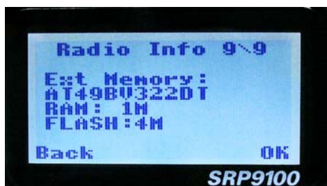
External Application Memory Status
