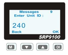
The entered digits can be deleted by using the ▼ key.
