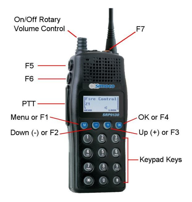
Figure 1 - SRP9130 Portable Key Layout
