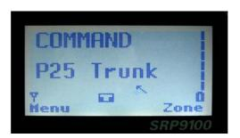
Trunked mode is indicated by the icon. The rotating arrow indicates that the radio is scanning for a trunked network. When the arrow is not shown, the radio is registered with the trunked network and ready to make or receive a call.
