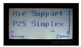
When stopped on a channel, the second line from the top shows the name of the channel from the scan group that the radio stopped on. If stopped on a channel, that channel can be "skipped" by pressing the skip programmed function key. Once a channel is "skipped" it will not be scanned for the duration that Zone/Channel selection.
