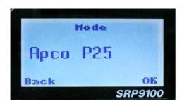
From the "**Mode**" menu, use the ▼ and ▲ keys to select the required operating mode, such as APCO P25, PMR or MPT Trunking. While the required mode is displayed, press OK to select that operating mode. The radio will then display the default screen for that mode.
