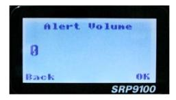
Use the ▼ and ▲ keys to change the relative alert volume level. The beep will sound at the indicated level each time the setting is changed.
