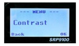
Press the "OK" key for the "Contrast" adjustment screen
