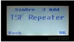
The second line from the top shows the name of a channel that is not a member of the Scan Group.
