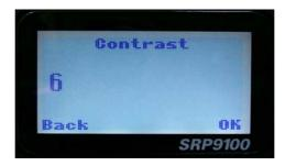
When the "Contrast" menu is selected, the contrast can be adjusted with the ▼ and ▲ keys. The numeric value of the Contrast is displayed.
