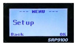
The ▼ and ▲ keys are then used to scroll through the setup menus.
