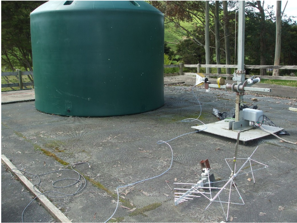
Radiated emissions test set up photos – Above 30 MHz
