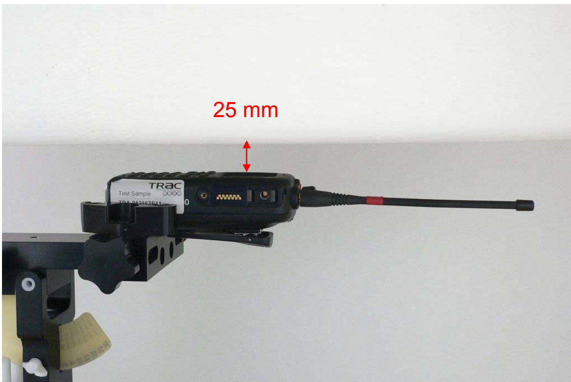
Fig. 15: Body worn configuration for the Simoco SDP660TU, PTT configuration with 25 mm distance, display towards the phantom.
