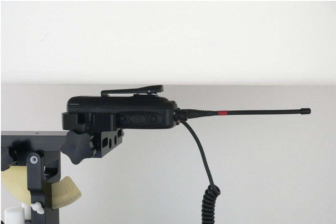
Fig. 14: Body worn configuration for the Simoco SDP660TU, PAR-600LMS4 remote speaker and belt clip attached, display towards the ground.
