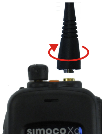
Figure 2. Fitting the Antenna.
