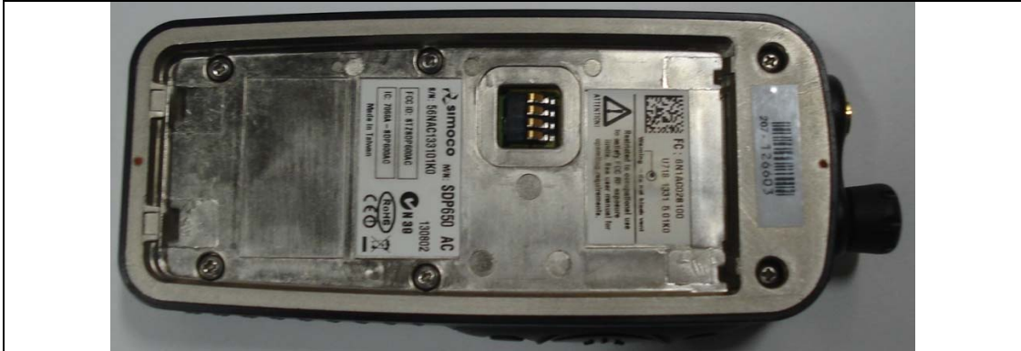
Back of DUT with Battery removed
