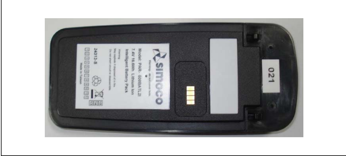
Back of Li-ion Battery
