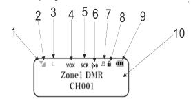
A signal icon resembling an antenna is on while the radio receives an RF signal. A 4-level bar graph to the right of this icon indicates the strength of the received signal. A strong signal will turn ON all 4 segments of the signal strength indicator bar.
