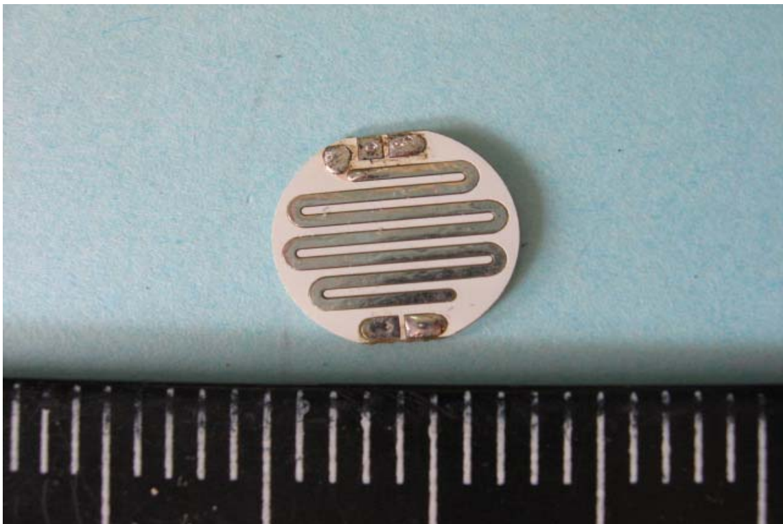
Solder View of PCB
