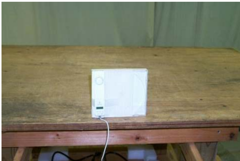
Figure 3.1 Radiated Test Setup-Position X
