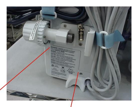
**GROUNDING:** Reliability can only be achieved when connected to an equivalent receptacle marked HOSPITAL GRADE.
