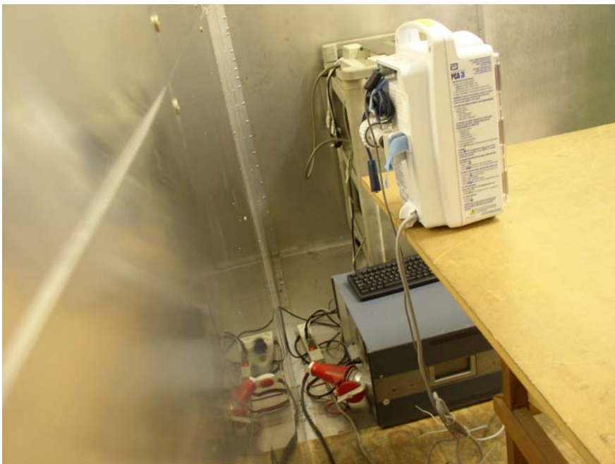
Conducted Emission - Side View
