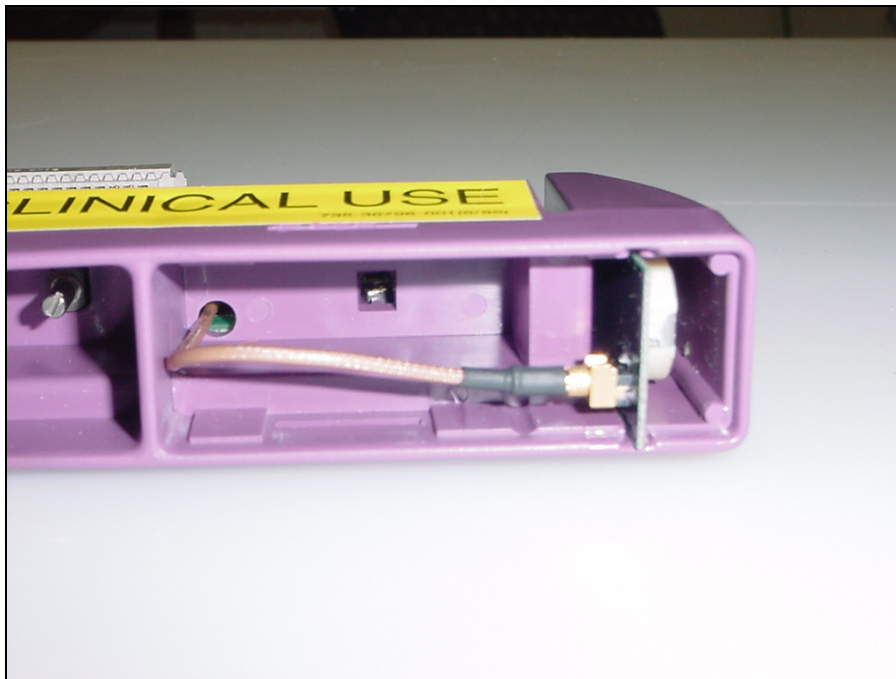
Photograph 5. Antenna mounted in housing
