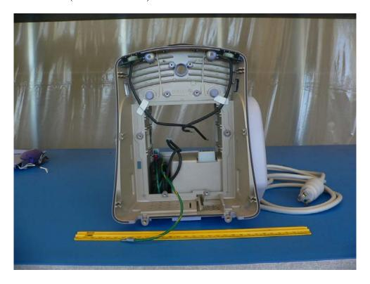
EUT Internal – Main Board with Microprocessor, PCB, Radio (Component Side View)
