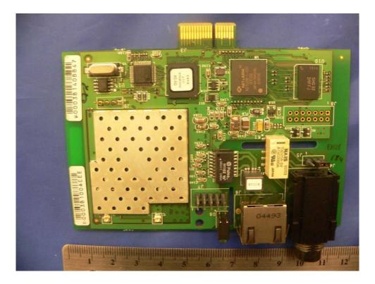
**EUT Internal – RF Board (Solder Side View)**
