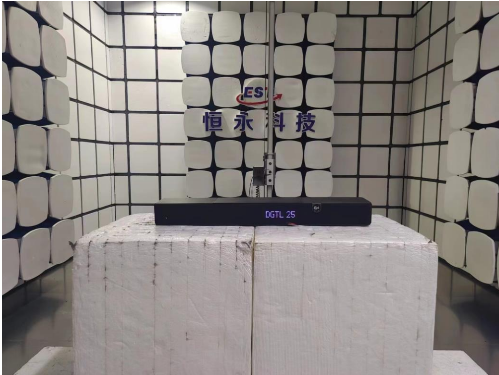
Radiated Test (Above 1GHz)
