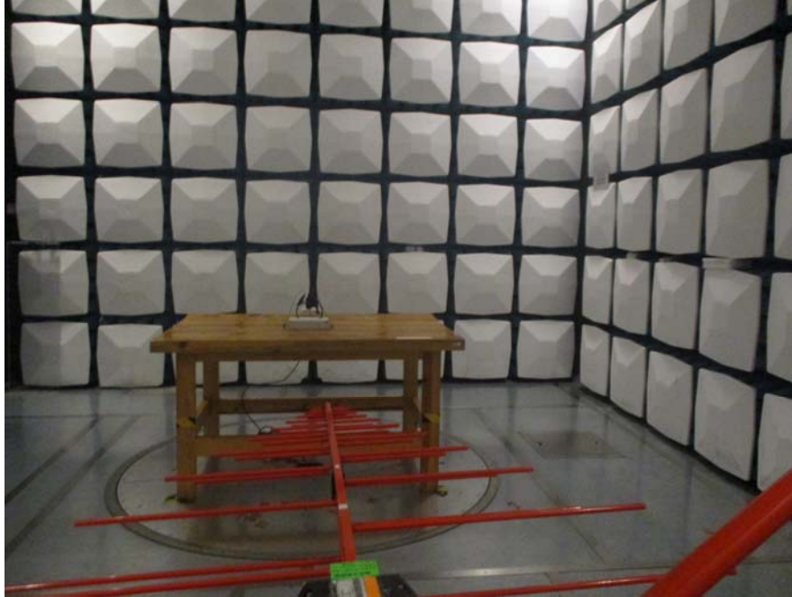
Radiated Emission View (Below 1GHz)
