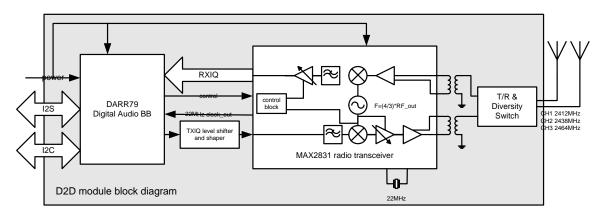
The D2D module can basically be regarded as a real time I2S to packetized RF converter.
