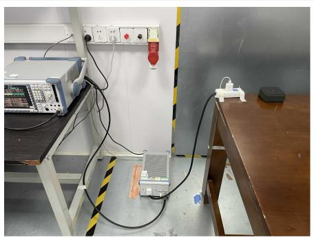
Conducted Emissions at AC Power Line (150kHz-30MHz)
