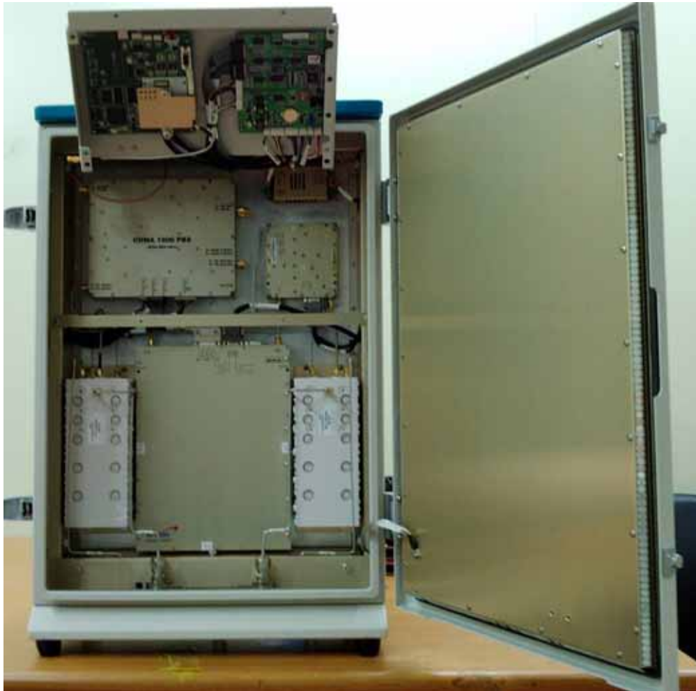
< The Inside of the Repeater>
