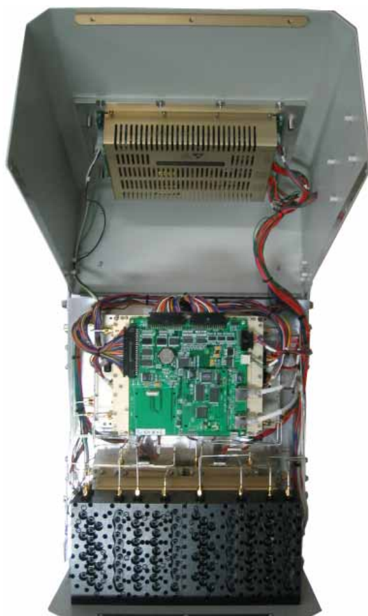
< The Inside of the Repeater >
