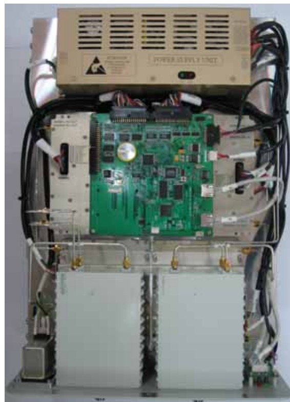
< The Inside of the Repeater >
