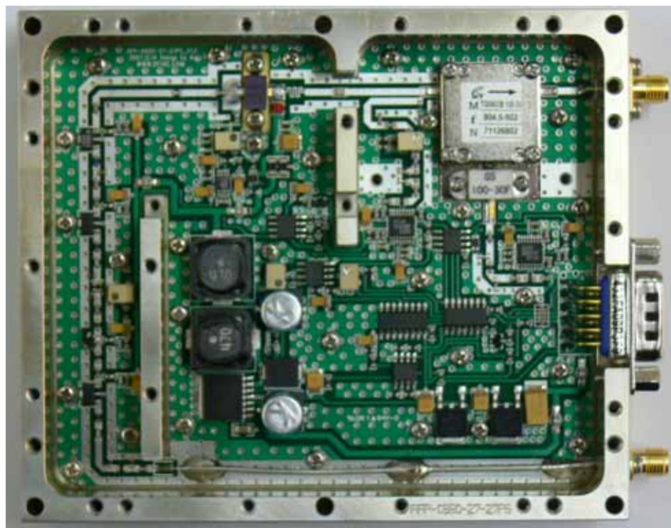
<RSN-iDEN-25-DC HPA Top View>
