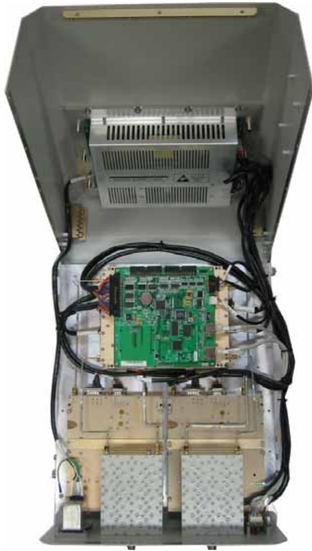
< The Inside of the Repeater >
