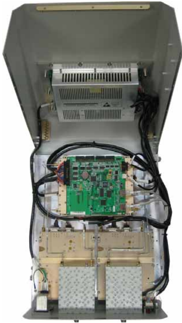
< The Inside of the Repeater >
