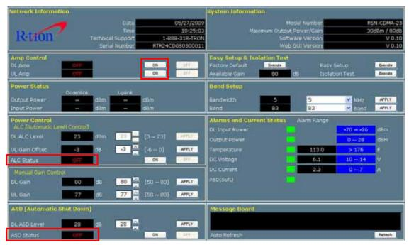
The maximum output power for operating is +23 dBm on both Tx and Rx.
