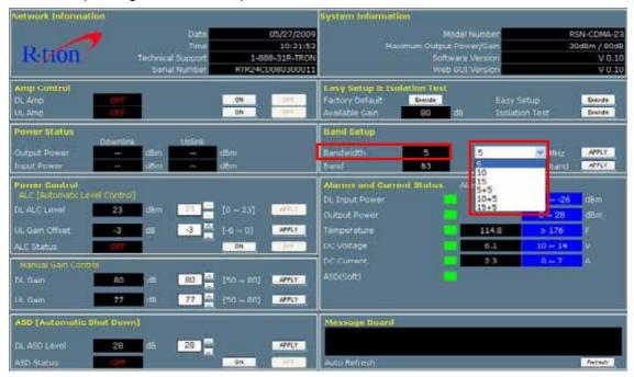
c. The operating frequency is able to be selected. Select the operating frequency and push the "APPLY" and check the bandwidth and frequency.
