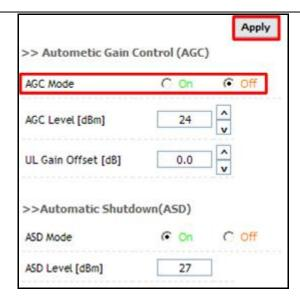
**Step 2.** The user can select any gain value as long as it does over-drive the amplifier or exceed isolation requirements. Gain is automatically limited where conditions do not permit high gain. Select the **DL** and **UL Fain values**. Turn on the **DL** and **UL path controls**.
