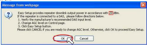
**Result.** Constant Maximum DL Output Power 20dBm (AGC Level 20dBm) If the DL input Power ≥ -71dBm
