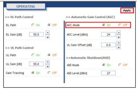
Step 5. Turn on the DL and UL path controls.
