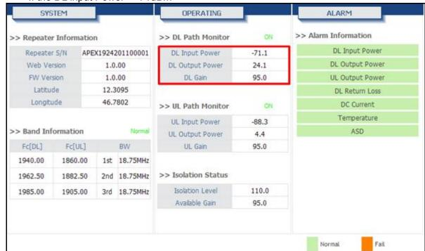
Result 2. Maximum Gain 95dB if the DL input Power <-71dBm
