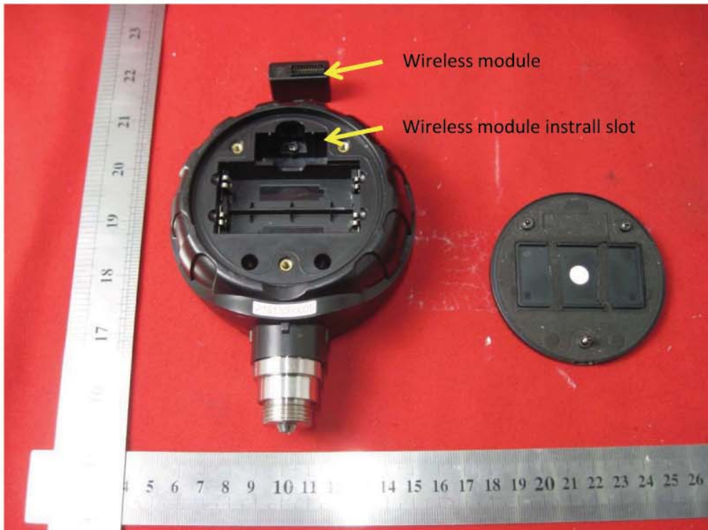
Rear side with removing the wireless module
