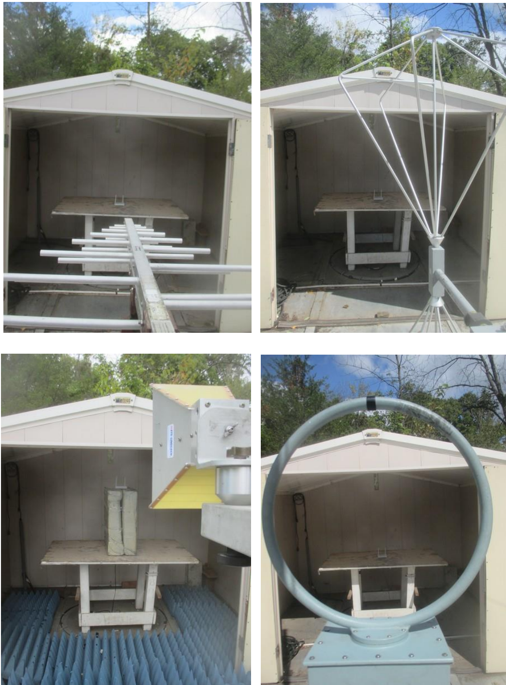
Figure 3.1 Radiated Test Setup
