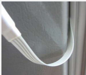
Ribbon cable easily slides through refrigerator door seal
