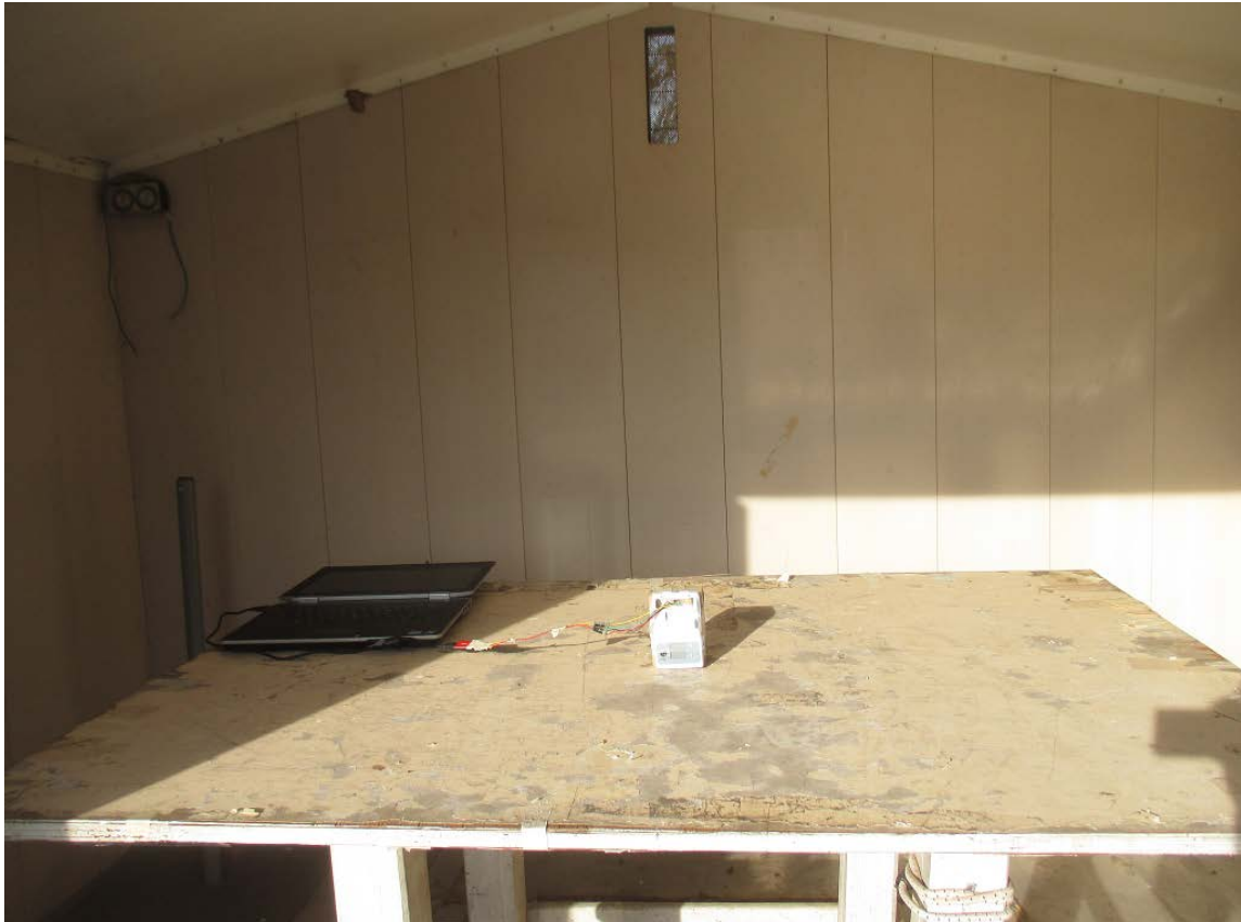
Figure 1 EUT Configuration for Radiated Emission Test (Button Up & Down)
