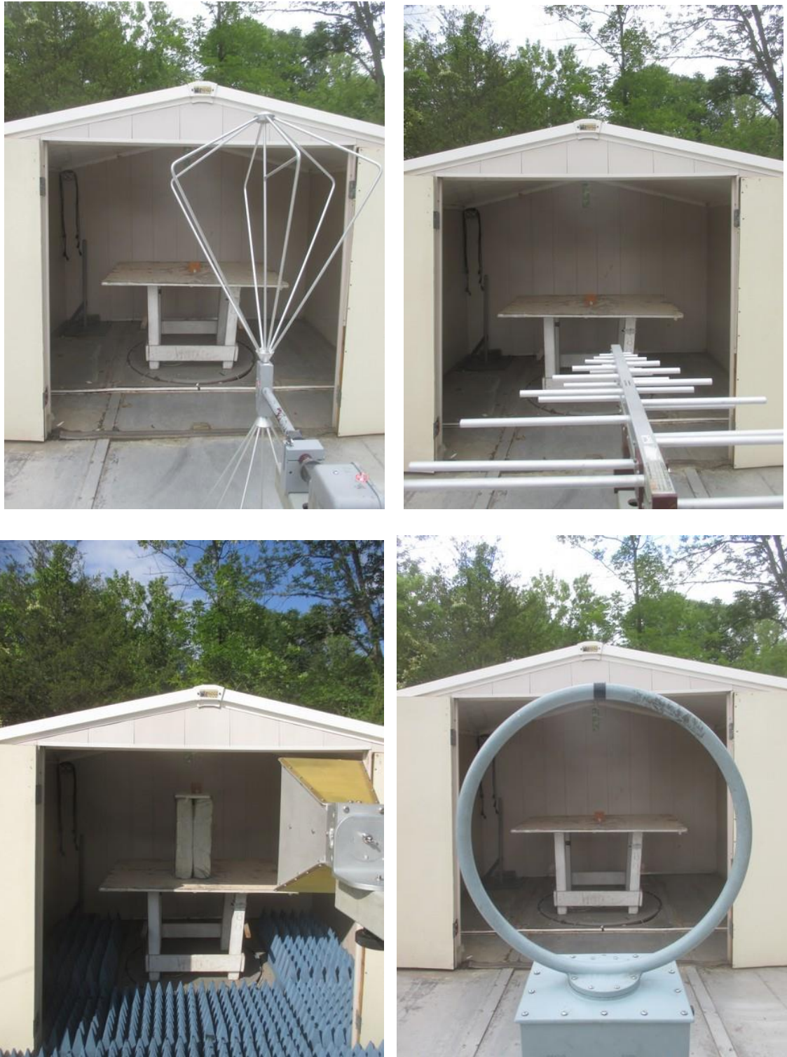
Figure 3.2 Radiated Configuration Test Setup
