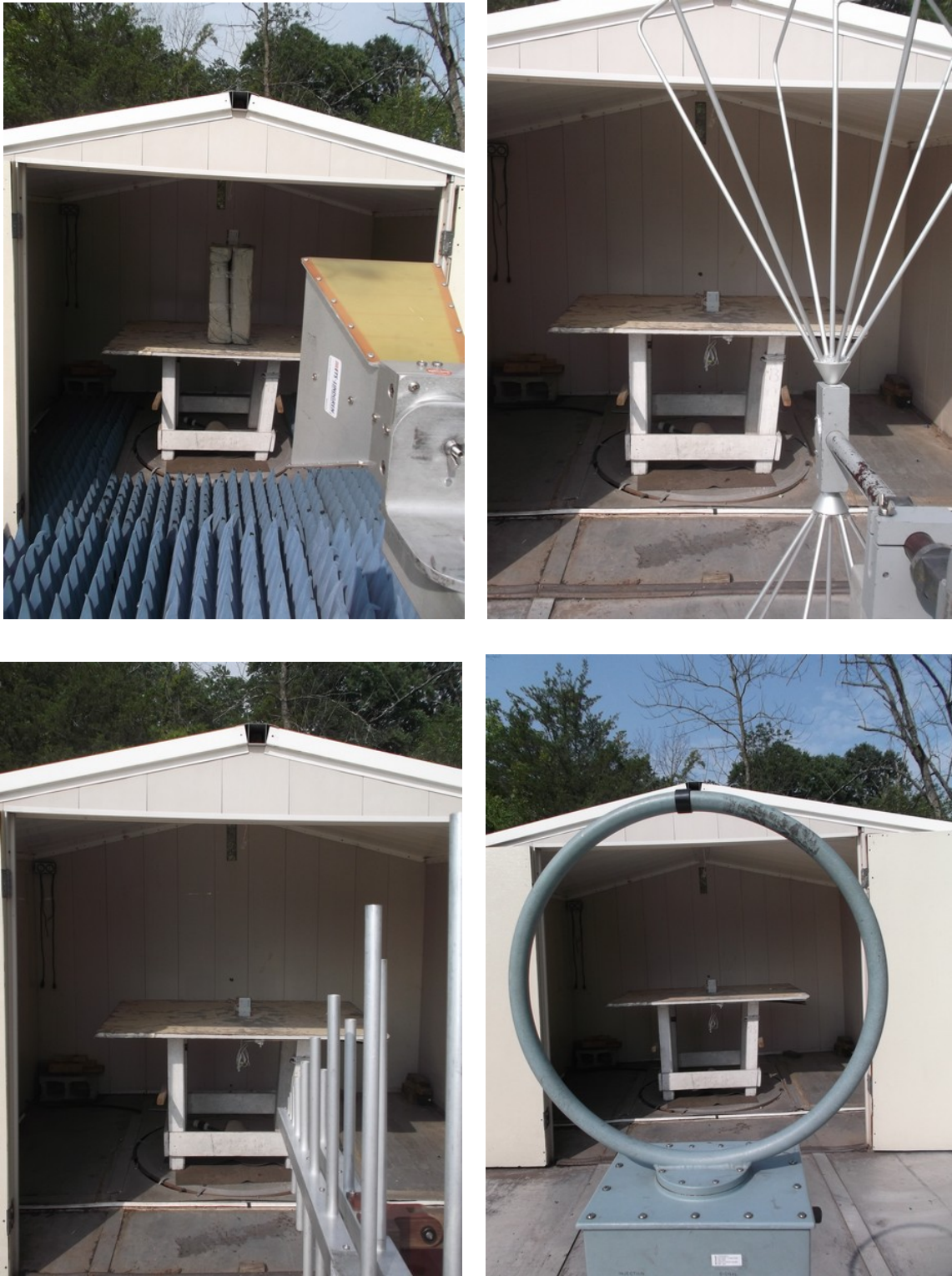
Figure 2 Radiated Emission Test Setup
