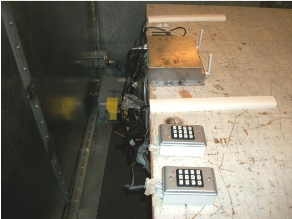
Figure 3.2 Conducted Test Setup
