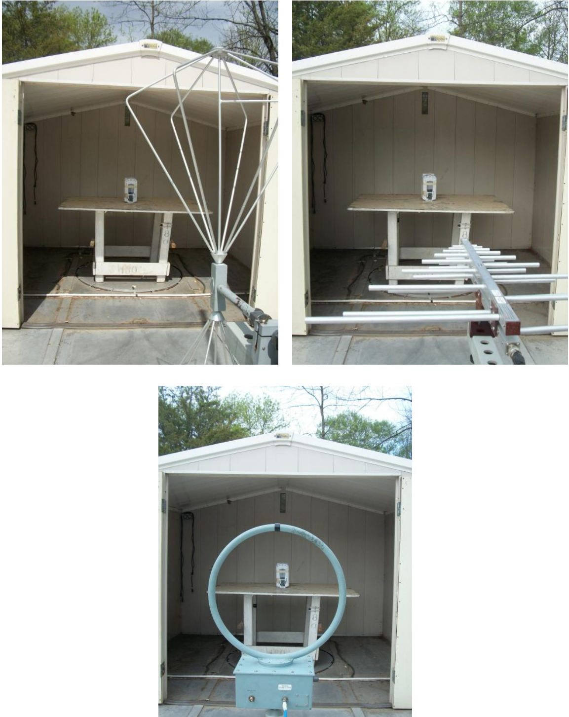
Figure 3.1 Radiated Test Setup
