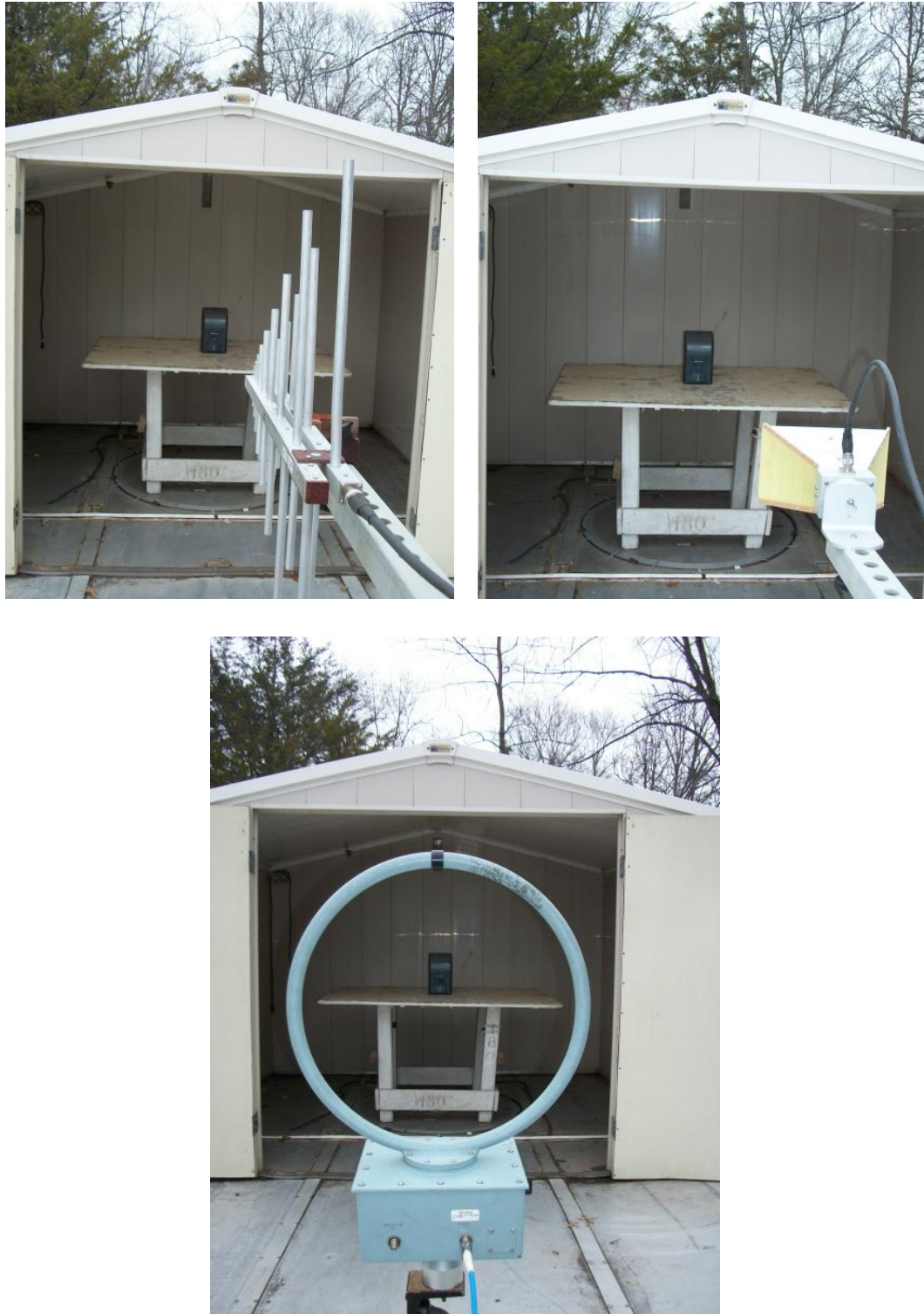
Figure 3.1 Radiated Test Setup
