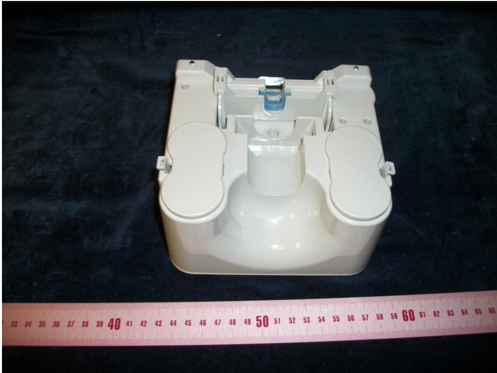
7.4 DC Battery Set Compartment
